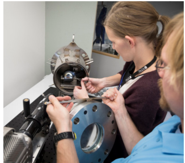
Nanostructured surface is mounted inside reactor for studies of CO 2 condensation at high pressure and low temperature
