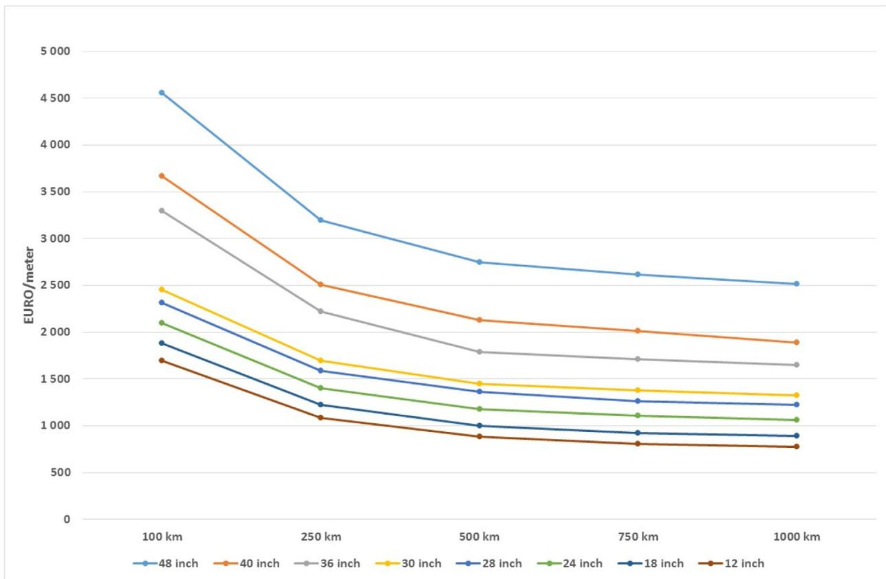
Fig. A1. Applied Pipeline cost in Euros/m and as function of diameter and distance as shown in Table A10.
