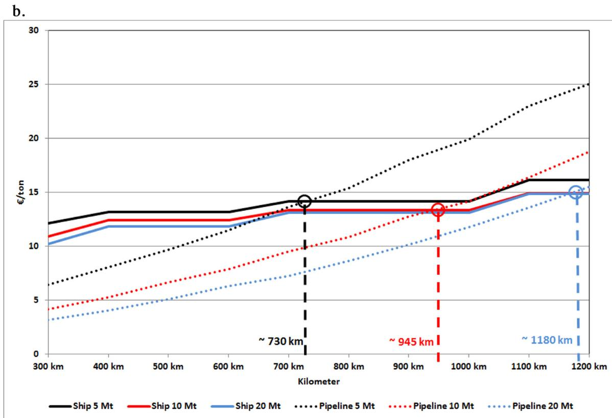
Fig. 2. (a) Comparison of ship and pipeline transport cost, €/t CO<sub>2</sub>, as a function of yearly transport volume and distance for transport volumes between 0.5 and 2.0 Mtpa.<sup>5</sup> as a function of yearly transport volume and distance for transport volumes between 5 and 20 Mtpa.
