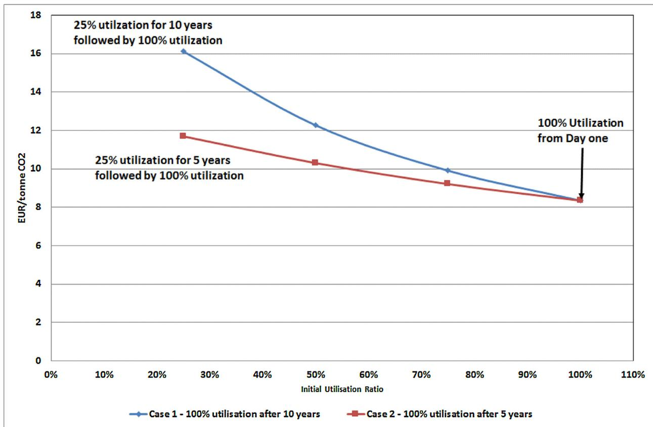
Fig. 4. Specific cost as a function of utilization ratio (25, 50, 75 and 100%) for a 500 km pipeline carrying 10 Mtpa CO<sub>2</sub> and reaching 100% utilization after 10 (blue line) and 5 (red line) years (for interpretation of the references to colour in this figure legend, the reader is referred to the web version of this article).
