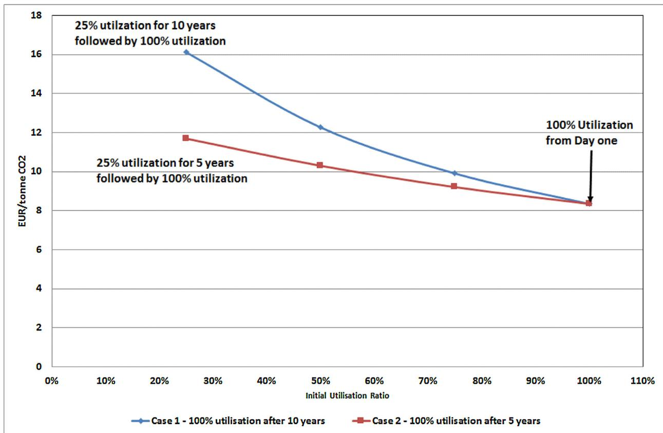
Fig. 4. Specific cost as a function of utilization ratio (25, 50, 75 and 100%) for a 500 km pipeline carrying 10 Mtpa CO<sub>2</sub> and reaching 100% utilization after 10 (blue line) and 5 (red line) years (for interpretation of the references to colour in this figure legend, the reader is referred to the web version of this article).
