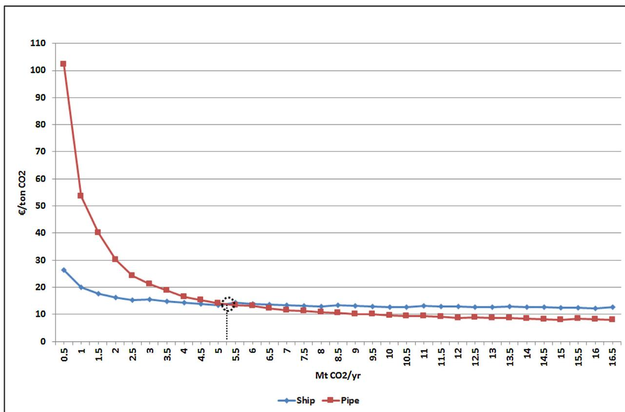
**Fig. 3.** Specific cost for transport by pipeline (red) or by ship (blue) as function of increasing volume of CO<sub>2</sub> from Östrands pulp mill in Piteå. The cost does not include cost for a collection or distribution system (for interpretation of the references to colour in this figure legend, the reader is referred to the web version of this article).
