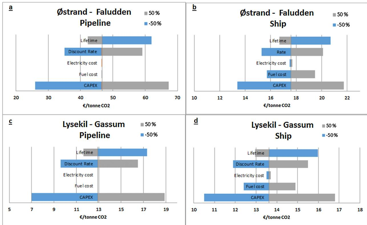
**Fig. 7.** The specific cost (€/t CO<sub>2</sub>) for pipeline and ship transport from Östrand to Faludden (case 2) and from Lysekil to Gassum (Case 6) as obtained from a 50% reduction and increase in lifetime, discount rate, cost of electricity, cost of fuel and CAPEX, relative to basic assumptions as specified in Section 2 (for interpretation of the references to colour in this figure legend, the reader is referred to the web version of this article).
