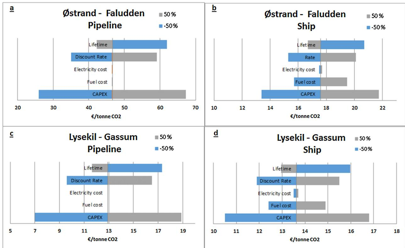
**Fig. 7.** The specific cost (€/t CO<sub>2</sub>) for pipeline and ship transport from Østrand to Faludden (case 2) and from Lysekil to Gassum (Case 6) as obtained from a 50% reduction and increase in lifetime, discount rate, cost of electricity, cost of fuel and CAPEX, relative to basic assumptions as specified in Section 2 (for interpretation of the references to colour in this figure legend, the reader is referred to the web version of this article).
