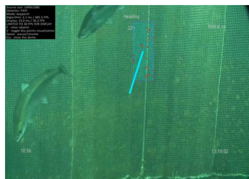
Figure 9 Automatic tracking of fish cage rope in camera pictures
