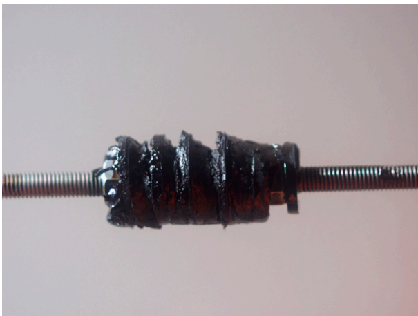
Wax deposits pigged out after an experiment without SATURN Cold Flow.
