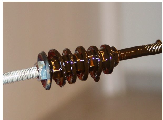
Pig with no wax deposits after an experiment with SATURN Cold Flow.
