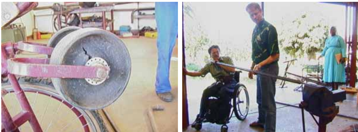
Photo: Damaged front caster and testing of materials. It is a huge need for guidelines and standards on materials, components, finished products and test methods
