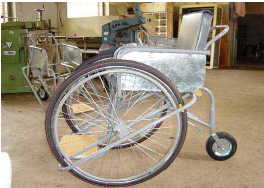
Photo: Huckstep Wheelchair being produced at Mulago Orthopaedic Workshop, Kampala
