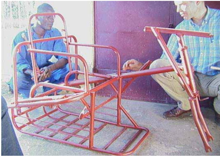
Photo: Tricycle and children wheelchairs being produced at Katalamwa Orthopaedic Workshop
