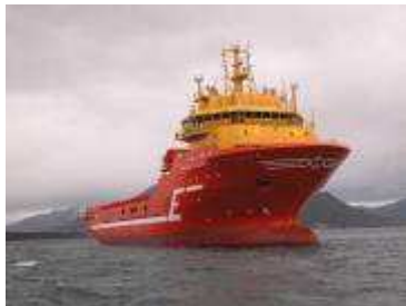
Viking Energy DF-electric offshore supply vessel Eidesvik Kleven Verft 4x 6R32DF 4x 49'500 running hours
