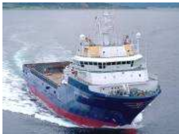
Stril Pioner DF-electric offshore supply vessel Simon Møkster Kleven Verft 4x 6R32DF 4x 46'500 running hours
