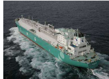
Provalys and Gaselys DF-electric LNG Carrier Gaz de France Alstom Chantiers de l'Atlantique 2x 12V50DF + 2x6L50DF Total 92'000 running hours for 2 ships
