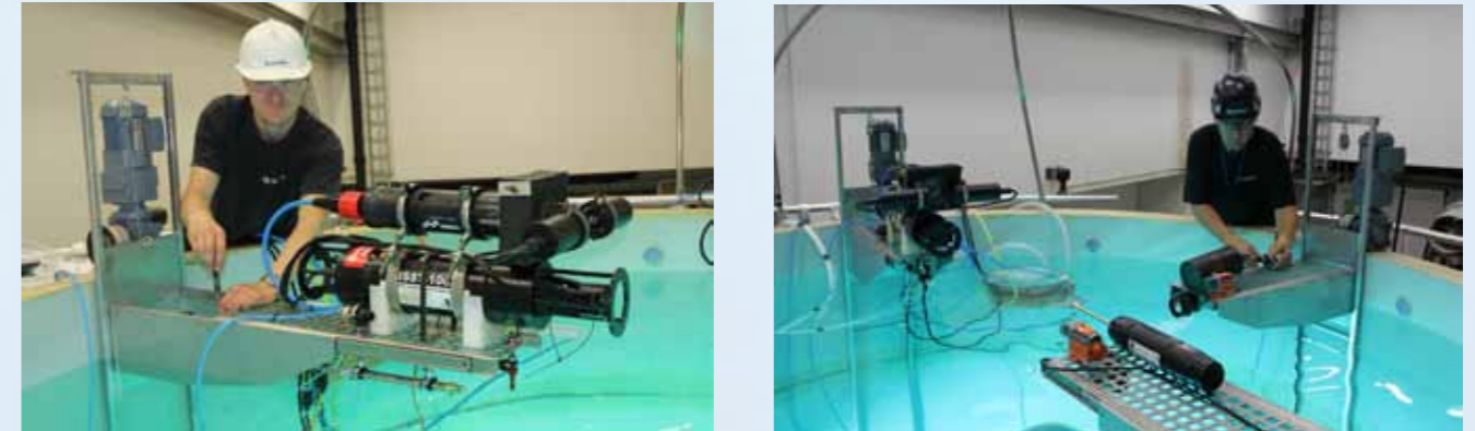
Figure 2: Pictures showing the main equipment used for monitoring of droplet sizes. Left: Mounting of laser scattering instrument (LIST100X) and the in-situ macro camera (close-up in figure 3). Right: Adjustment of camera equipment and the Vitrino 3D current profiler with all three instrument platforms in surface position.
