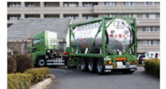
Truck with direct contact latent TES trailer, Japan
