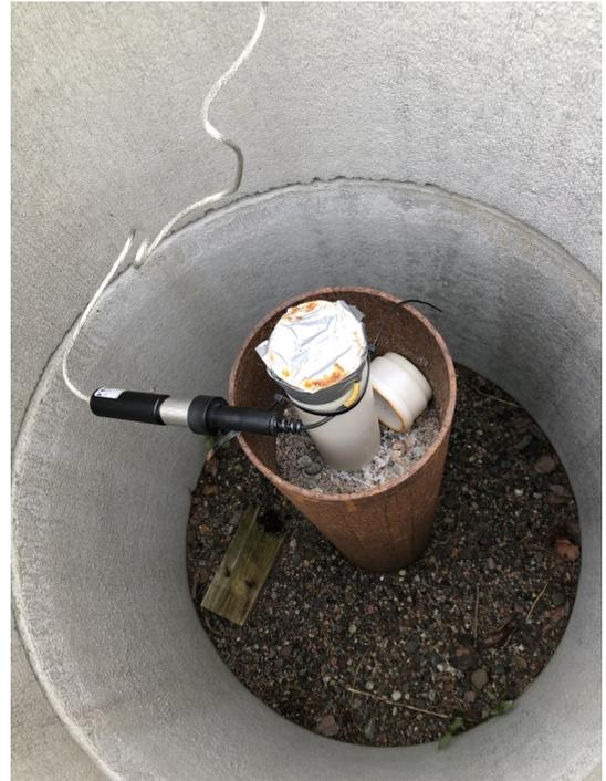
Readout of data from water level monitoring probe in one of the shallow wells at the site.
