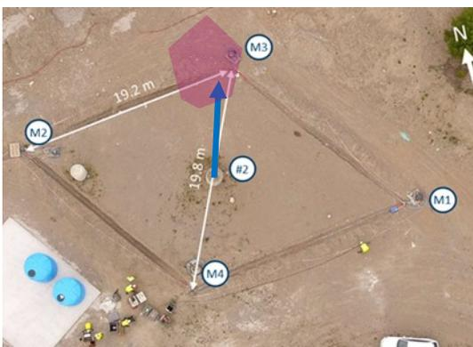
Approximate surface location of the CO<sub>2</sub> plume around well M3 during injection experiments.
