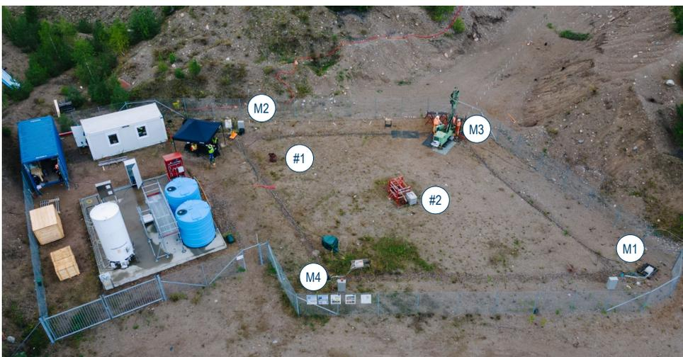
The distance between the injection well (#2) and the monitoring wells M4/M3 is 9.9 m. The distance is 16.7 m for M1/M2.
