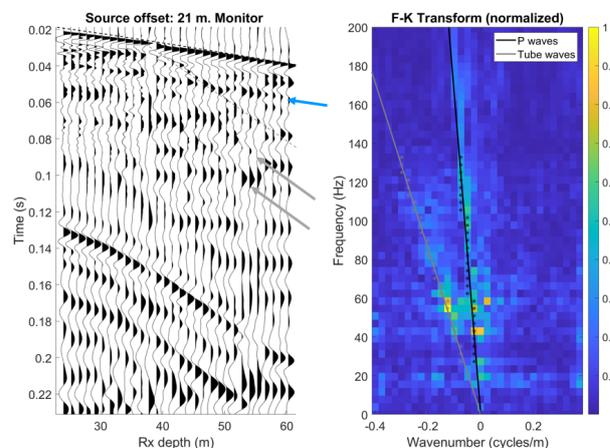
Example data showing tube waves that can be used for detection of CO<sub>2</sub> on the outside of the casing of well M3.
