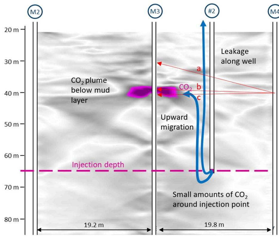
Several injection campaigns, conducted since 2019, show the same site behaviour and CO<sub>2</sub> migration when CO<sub>2</sub> is injected: The CO<sub>2</sub> migrates upwards from the injection point and accumulates as a CO<sub>2</sub> plume around well M3 below a mud layer at ~37 m depth. In addition some leakage (~10% of the injected amount) is observed along the outside of the injection well casing. The acquired seismic data shows exceptional data quality and repeatability.
