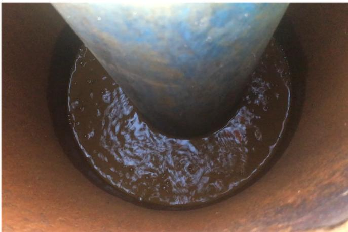
Leakage (CO<sub>2</sub> bubbles) observed along the outside of the injection well PVC casing (blue).
