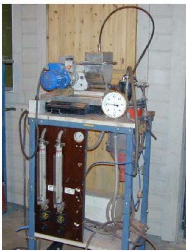
Figure 6: Erosive wear test apparatus no. 1
