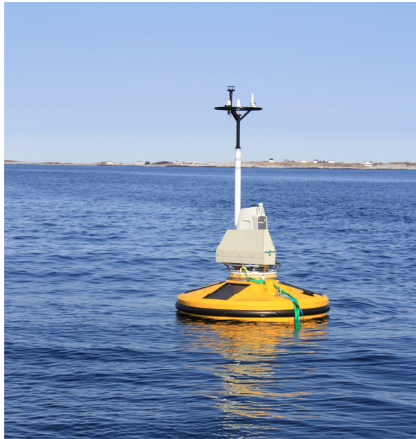
Figure 7. The Wavescan buoy with the ZephIR lidar off Titran
