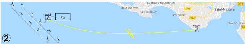
② CS2: Connected - Offshore Wind Farm – Offshore Electrolysis
