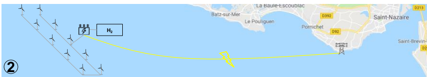
CS2: Connected - Offshore Wind Farm – Offshore Electrolysis
