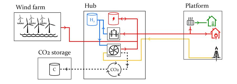
with wind power as the main energy supply can eliminate or greatly reduce CO<sub>2</sub> emissions.
