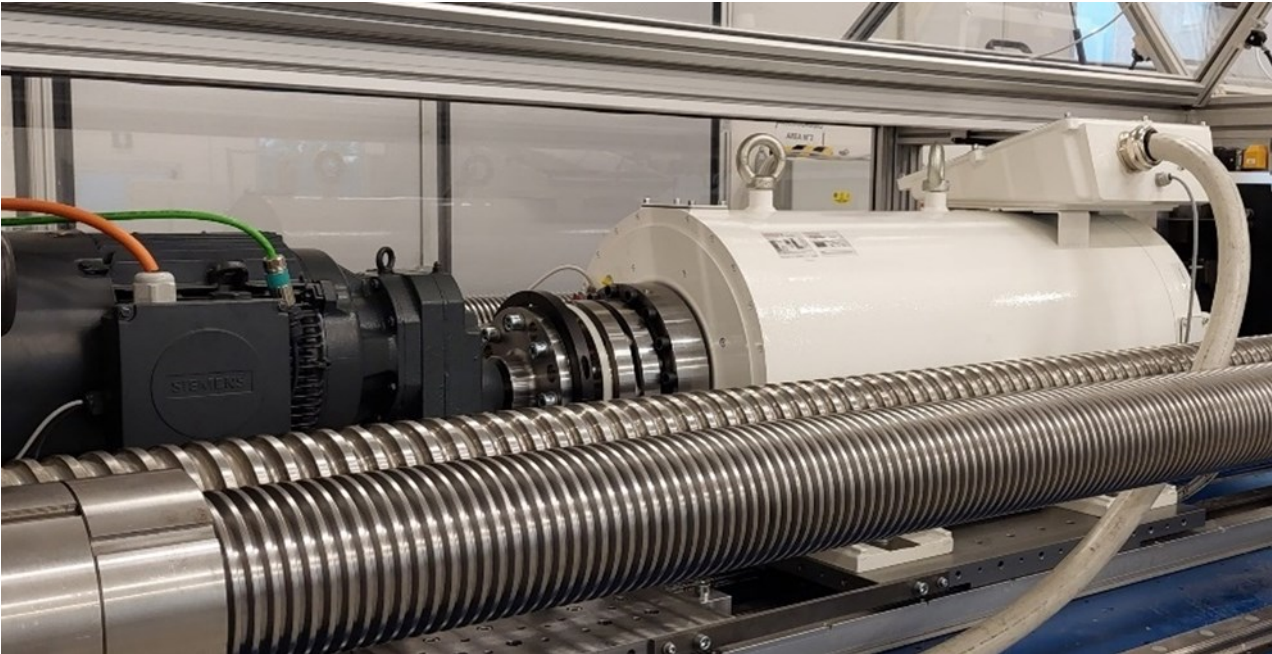
Figure 15 The actuating motor (machine on right-side) connected to a geared generator on the drivetrain test rig at VGA facilities.
