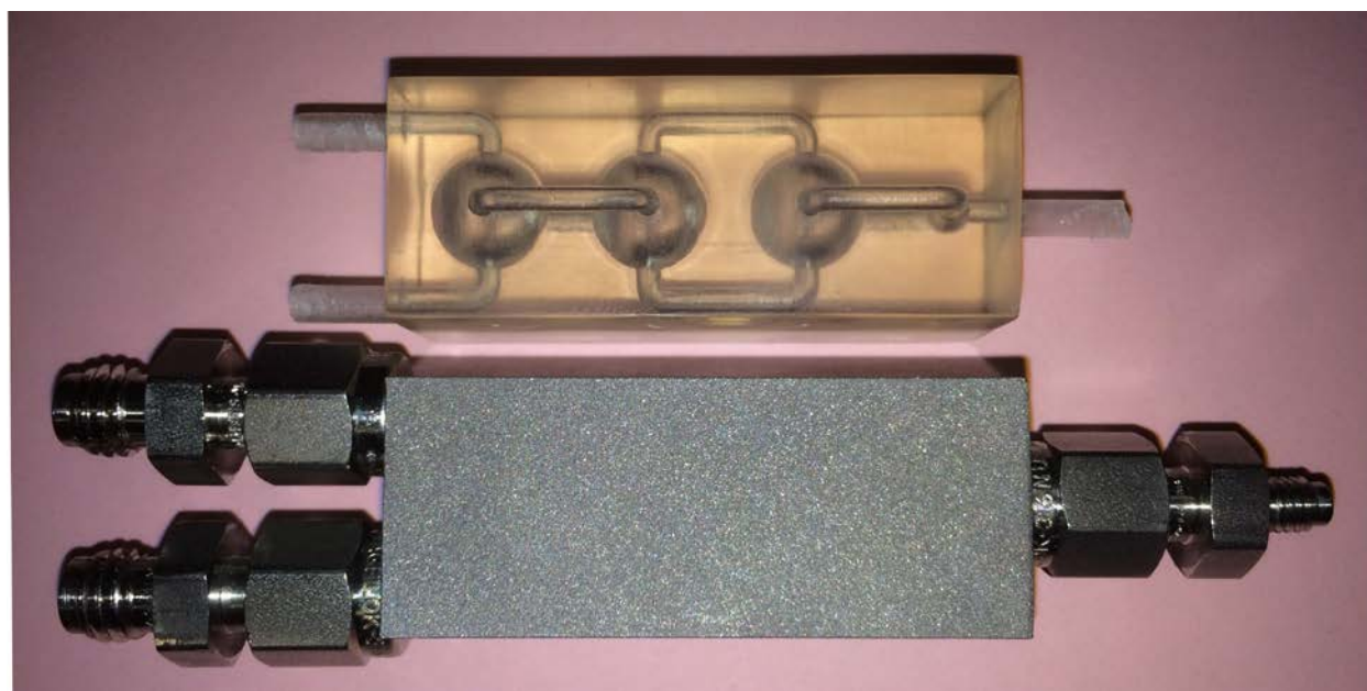
Fig. S2. Prototype and metal reactor used to continuously produce H-KUST-1 metal-organic framework.
