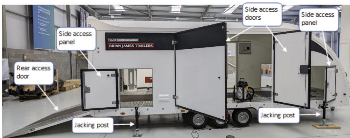
Figure 10: HD HFTS Trailer with access doors and panels open.
