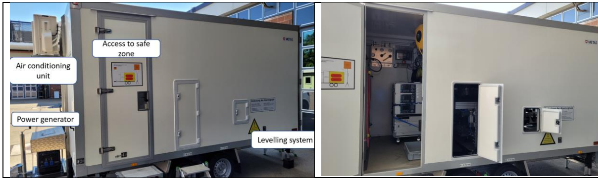
Figure 7: Left) Side view of the trailer, Right) same as left but with doors open.
