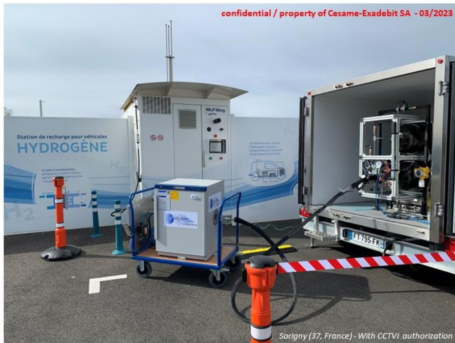
Figure 11: The CESAME Rover connected to the CESAME primary standard at the Sorigny (37) HRS.
