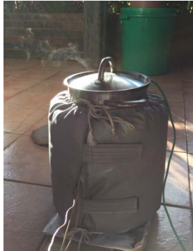
PCM bean cooker from excess PV power (Tanzania)
