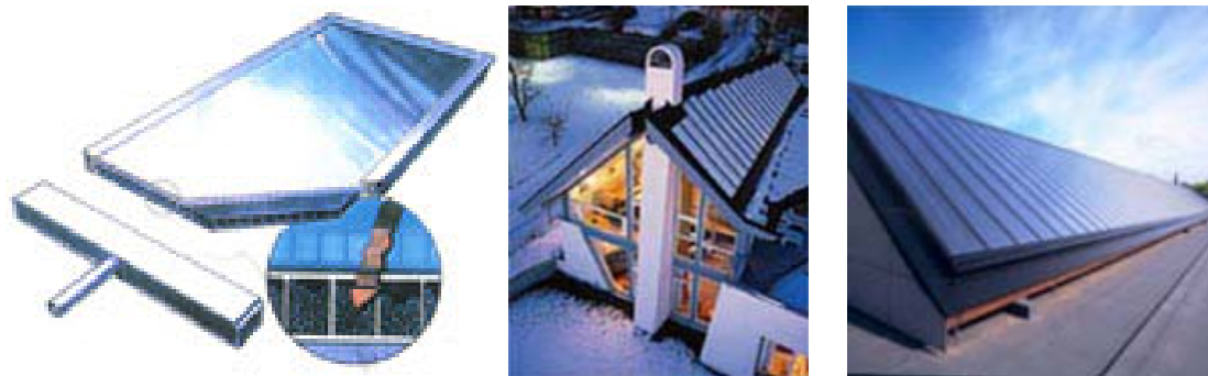
Figure 2-7 The SolarNor solar thermal collector is composed of a transparent sheet of polycarbonate plastics covering a black double sheet made out of the plastic material noryl. The inner structure is composed of narrow channels filled with small, porous pellets. Water trickles through a channel structure, absorbs the heat which is deposited in the absorber and carries the heat to a heat store.
