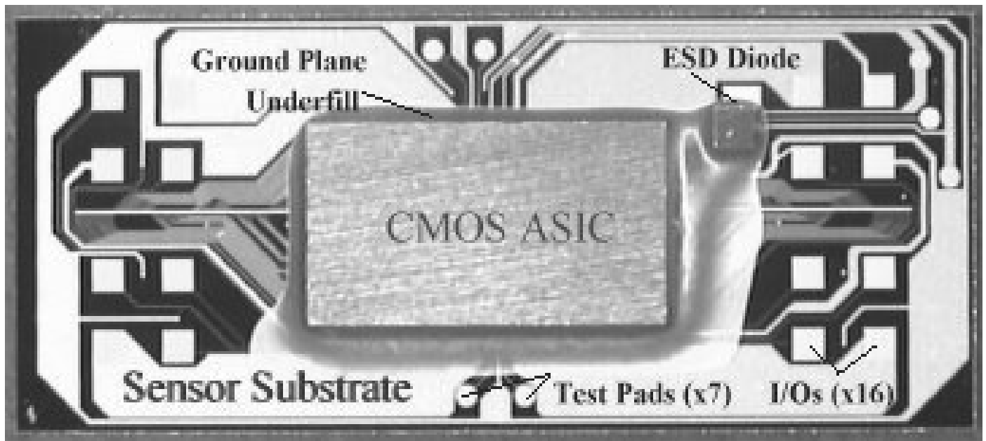
Figure 12.2.5: Module backside micrograph.
