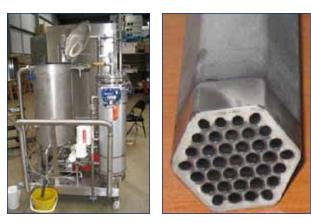
*Left: Pilot unit for application testing of the Watercatox process. The unit has 0.3 m<sup>2</sup> contactor area and >300 L/h capacity.*
