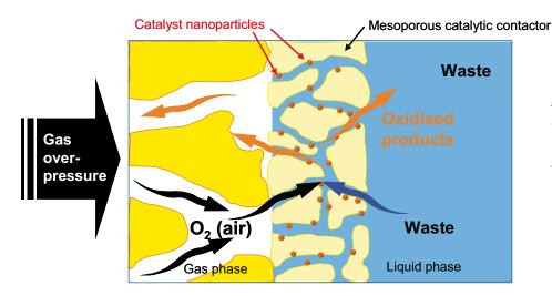
An overpressure of air or oxygen is applied to the outside wall of the tube. The overpressure (5-15 bar) forces the gas-liquid interface to a position close to the catalytic layer.
