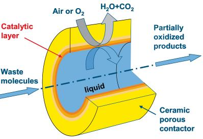
Principle of operation of the Watercatox process. The porous contactor tube has a layer on the inside wall containing catalytic nanoparticles where the oxidation takes place.
