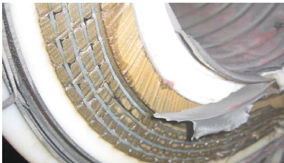
Figure 20: Un-bonded flexible riser with external fire protection layers and 4 tensile armour layers [75]
